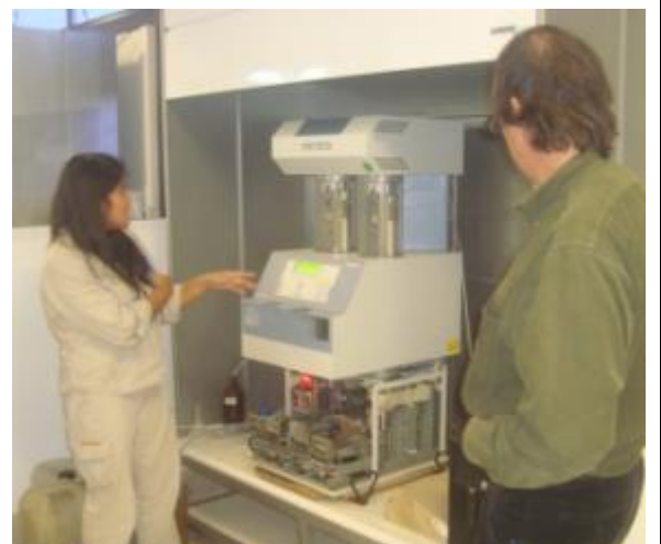
Picture 11 Ing Jorge Hilbert hearing the explanation of the quality laboratory member about an Herzog's HVM 472 Automated Multi-Range Viscometer.
